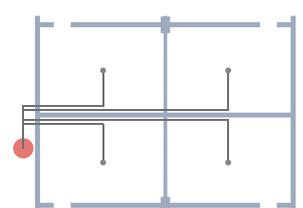
VSN 1230 fire extinguishing systems can be designed for use as a single-zone system to protect a single protected area or in the form of a multi-zone system to protect two or more areas.
